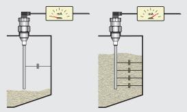
Measurement of electrically non-conductive materials:
